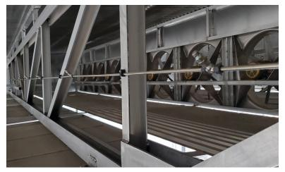
Another reason for Nyle's Atomizing Spray System is for wood conditioning. During wood conditioning, moisture is added back to the surface of the wood at the end of the drying process to help reduce any stresses in the wood from the drying process.
